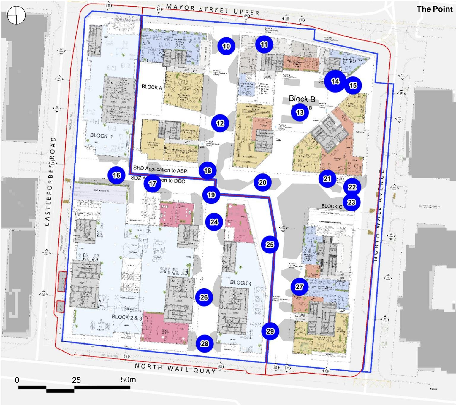
We have calculated the Level of Service (LoS) as per the Fruin guidelines at the location with the narrowest width within the SDZ and SHD developments.
