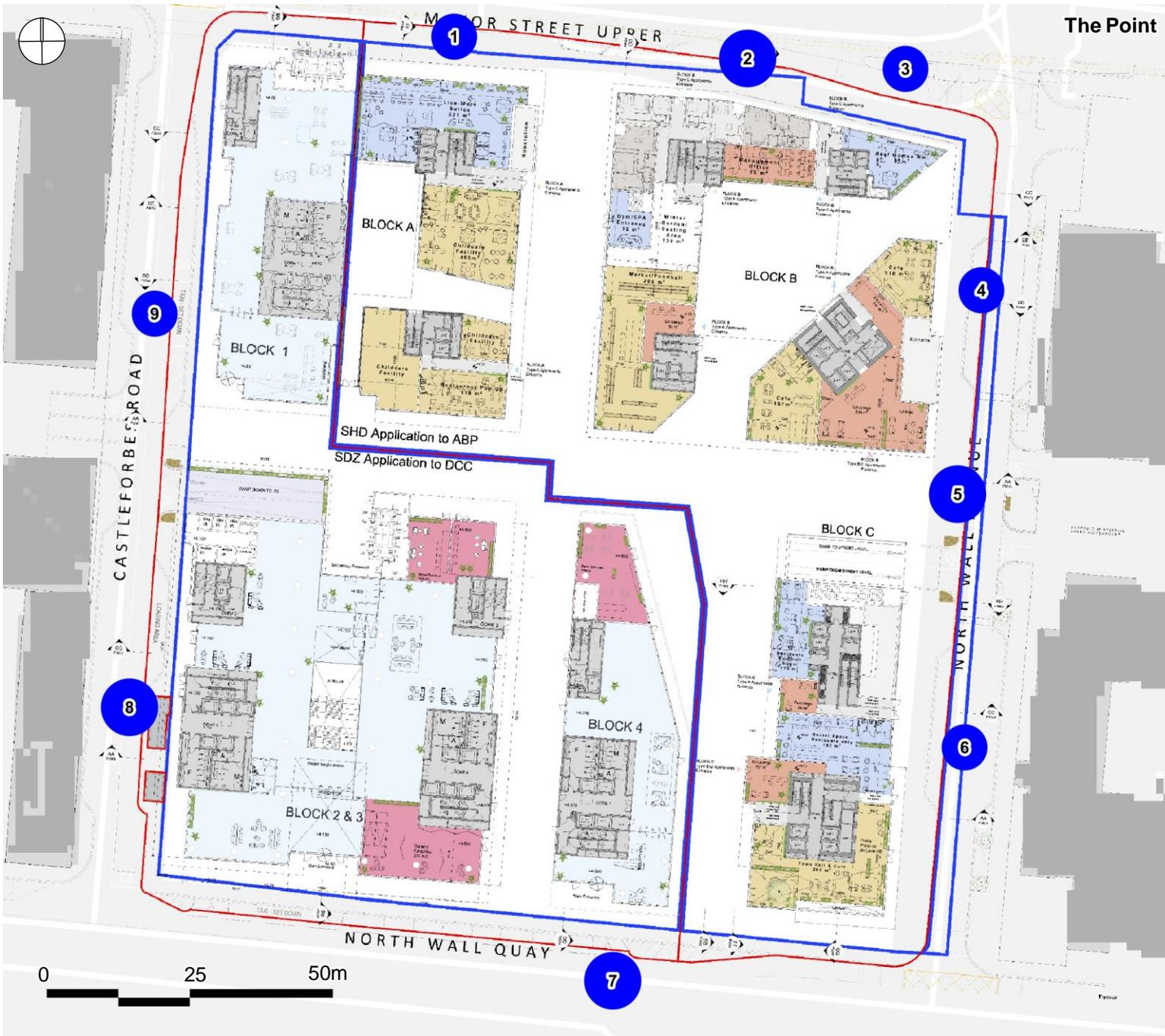
We have calculated the Level of Service (LoS) as per the Fruin guidelines at the location with the narrowest width along the external pavements.
